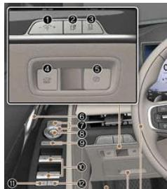
① In the case of an automatic transmission vehicle, press the P button with the brake pedal pressed to activate the vehicle parking mode.
