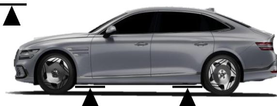
To stabilize the vehicle, crib at four points directly under the front and rear pillars using wooden blocks or equivalent objects
