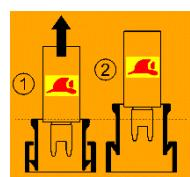
④ Open the fuse box cover wearing a fire-proof helmet and pull up the high voltage cut-off switch
