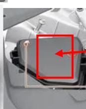
③ The high voltage cut-off switch is in the fuse box
